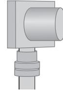
**The Temperature Sensor** monitors the exhaust air temperature in the duct. A signal is transmitted to the I/O Processor to vary the fan speed in proportion to the actual heat load. (To optimize energy savings and kitchen comfort, additional temperature sensors can monitor the outside air and kitchen space temperature.)
