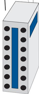
**The I/O Processor** controls the lights and/or fans for up to four hoods. It is typically mounted in an end-cabinet, and communicates between the hood sensors and Electronic Motor Starter(s) via plug-and-play cables (RJ-45). It is also connected to the Keypad mounted on the front face of one of the hoods for easy user interface.
